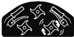
Clutch disengaged      Clutch engaged
