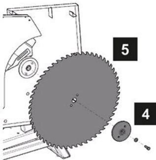
9- Remove the locking tool and put back the protective casings
