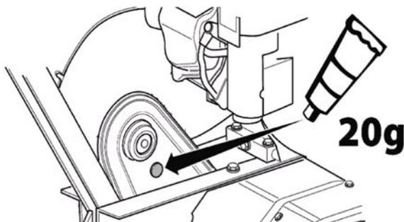
1- Remove the cap from the upper part of the transmission
