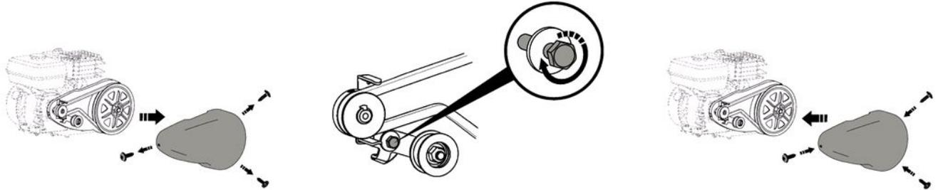
1- Remove the 3 belt cover holding screws
